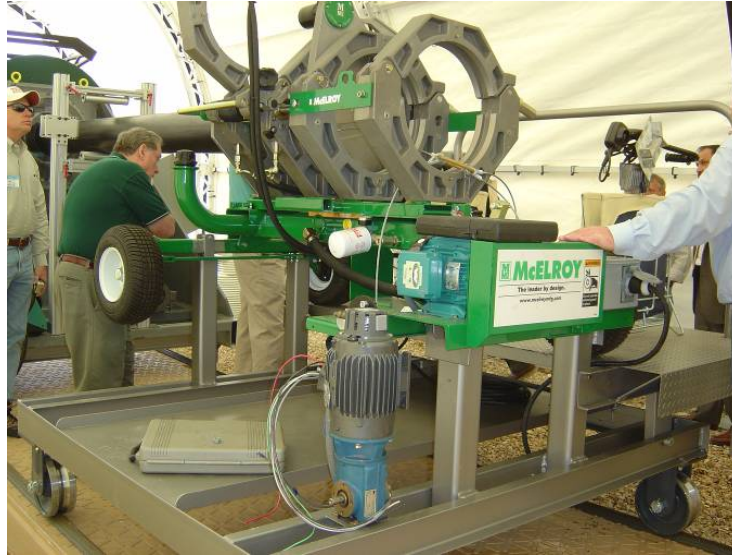
Figure 2. - Welding the HDPE Core Pipe
